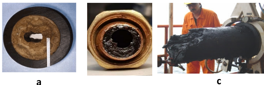
Figure 2: Sample of wax deposit; (a) (Singh et al. 2000) and (b) (in-house) decreases in the actual pipe diameter (c) completely blocked pipeline system (Ricky 2016)
